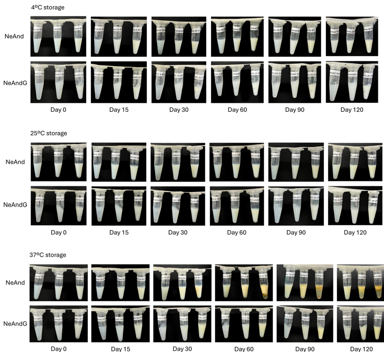
Figure 2. Effect of temperature and time of storage on the macroscopic aspect of andiroba oil nanoemulsion (NeAnd) and its gel form (NeAndG). Each image contains three eppendorf tubes in the following sequence: NeAnd 10, 20, and 40 and NeAndG 5, 10, and 20. Samples were stored at 4, 25, and 37 °C for 120 days under light protection, and the pictures were registered on days 0, 15, 30, 60, 90 and 120.
