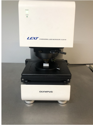
Figure 3.7: Olympus LEXT OLS4100 confocal laser microscope [58].
