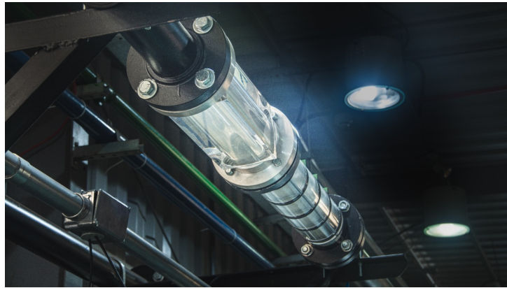
Figure A.8 – Two-phase test bench: (a) schematic with distances between resistive sensors, and (b) a photo of the experimental setup highlighting the visualisation section and the void fraction sensor.
