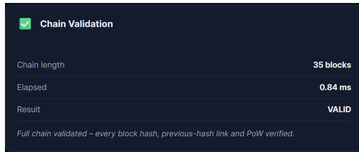
Figure 5.7 – Blockchain chain validation result confirming that all blocks have valid SHA-256 hashes and correct previous_hash linkage.
