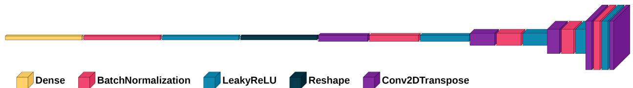
Figure 3.6: Block diagram of the convolutional layers in the GAN generator model used (Dense, BatchNormalization, LeakyReLU, Reshape, and multiple Conv2DTranspose layers and Conv2DTranspose layer).
