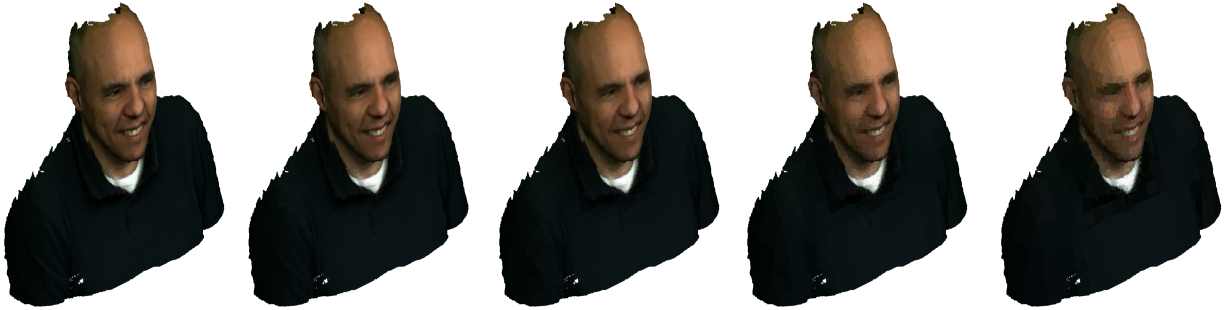
Figure 3.5: Illustration of projections of the point cloud sequence “Ricardo” decoded using SPIHT, and cutting the bit stream at different bit-planes. From left to right: original (14 bit-planes), 11 bit-planes, 10 bit-planes, 9 bit-planes, and 8 bit-planes.
