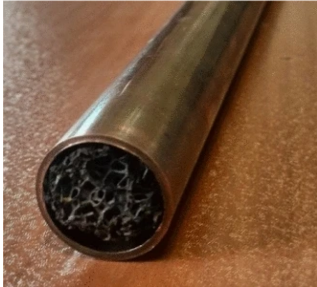
Figure 1.4: Pipe filled with porous metal foam. (Amani et al. [1])
