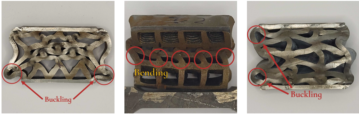
(a) Diamond pattern local buckling in several struts. (b) Square pattern deformation mainly governed by strut bending. (c) Triangle pattern pronounced local buckling, especially near boundaries.
