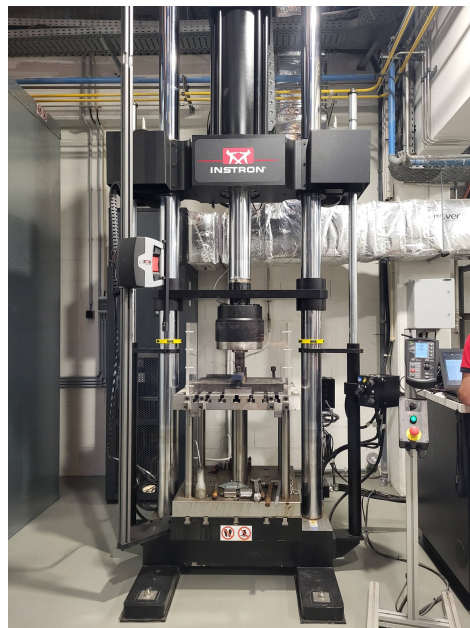
Figure 3.4: Instron 1000HDX universal testing machine used for the tensile destructive test. Provided by INEGI.
