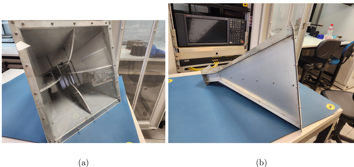
Figure 3.10: Manufactured square quad-ridge horn antenna: (a) a diagonal view, and (b) a side view.
