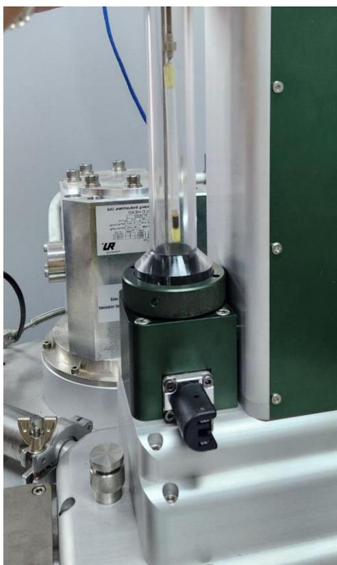
Figura 10 Amostra CoFFee no magnetômetro SQUID.
