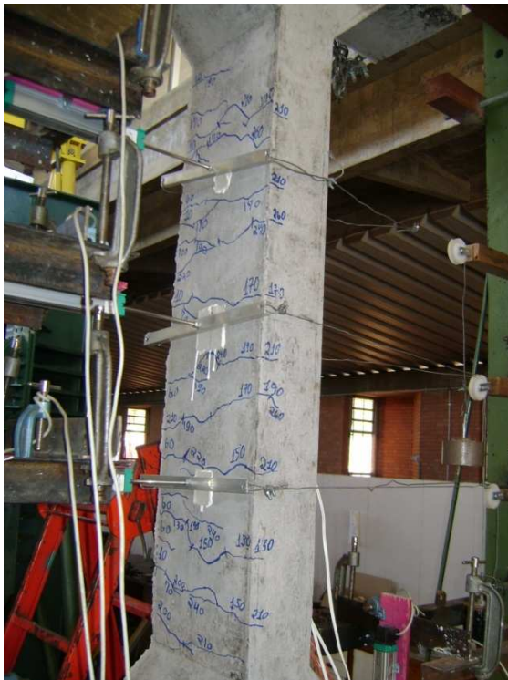
Figura 4.10-Fissuras no Pilar PFN 40 - 2,0
