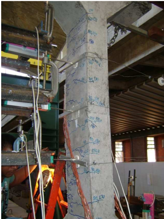
Figura 4.14-Fissuras no Pilar PFN 60 - 2,0
