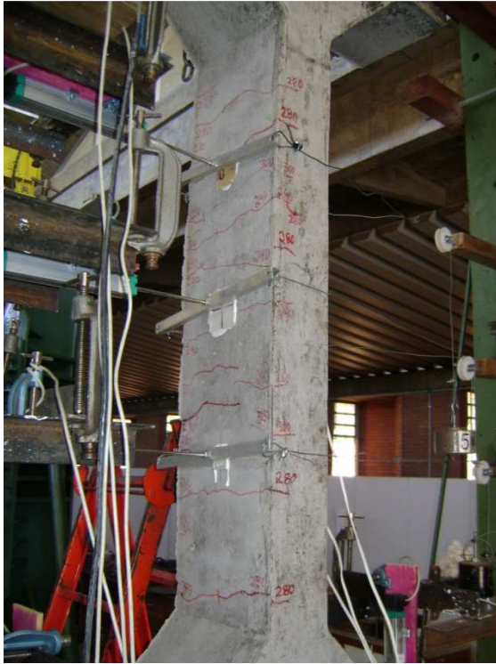
Figura 4.8 - Fissuras no Pilar PFN 30 - 2,0
