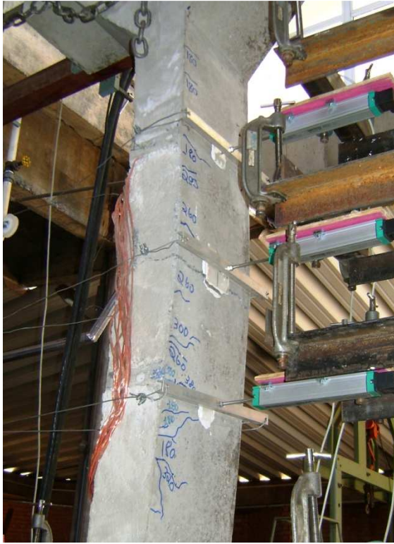
Figura 4.4 - Fissuras no Pilar PFN 15 - 2,0
