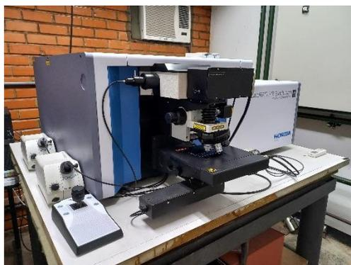
**Figura 38: Espectrômetro Raman, LabRam HR Evolution do NFA.**
