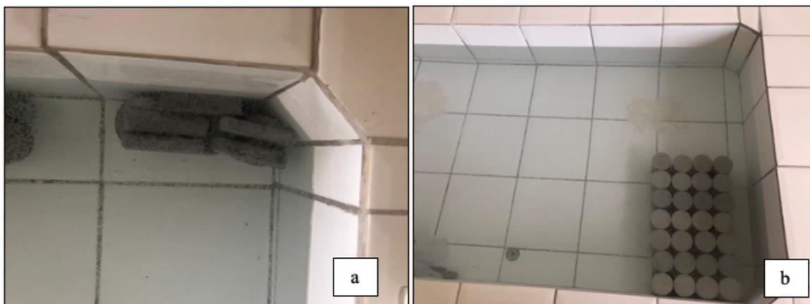
Figura 3.24- Aspecto dos CdP's no tanque de cura: (a) CdP's 20 x50 mm; (b) CdP's 50 x100mm.
