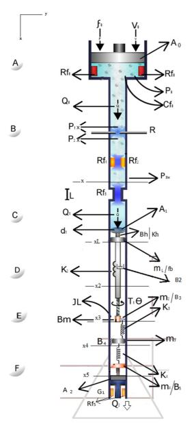
Figure 2. Mechanical and hydraulic representation analogous to the esophagus system, and its variables and constants.
