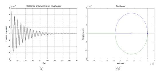
Figure 6. (a) Response of the system modeled to the impulse signal; (b) Root-Locus of the system modeled. Note that the eingevalues are in the left semi-plan providing stability to the system.
