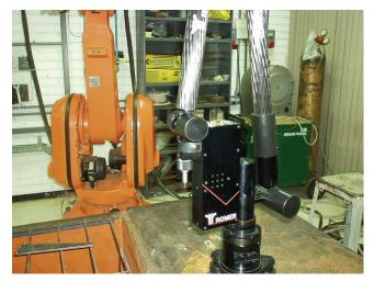
Figure 4. ITG ROMER measurement arm.
