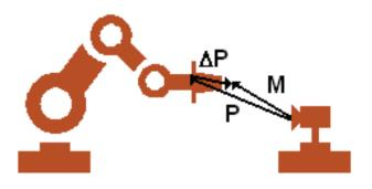
Figure 6. Simplified representation of the calibration transformations.
