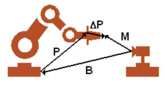
Figure 5. Calibration transformations.
