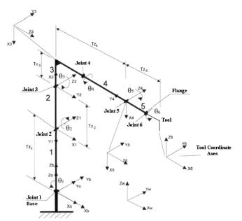
Figure 2. Kinematic Model of the IRB-2000 robot.
